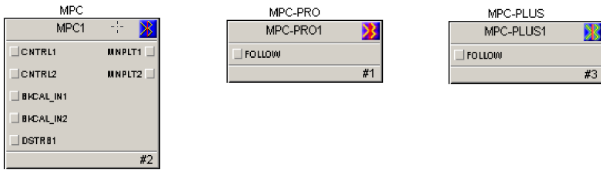
Figure 3-3: MPC blocks in DeltaV
